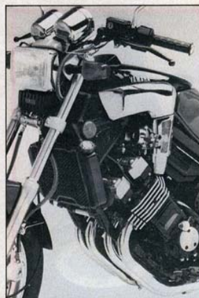
The area around the steering head is cluttered with various hoses and screens, and the radiator looks too wide for the rest of the bike.
