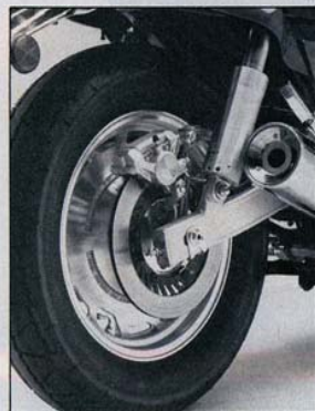
The shocks resemble the once-popular Fox Airshox, but they're actually just upside-down deCarbon dampers with covers over their coil springs.
